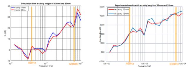
Figure 10: Comparison of IL evolution between experimental results (right) and simulation (left).
