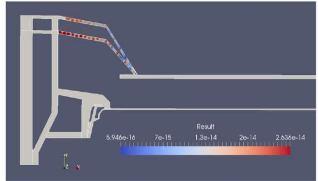
Figure 13: Y displacement distribution at 4000Hz for a cavity length of 37mm and 47mm.
