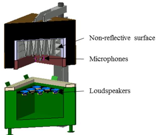
Figure 2: Cross-section of the CAD model of a small cabin.
