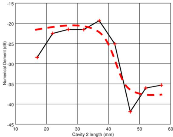
Figure 11: Demerit evolution for a variation on cavity length.
