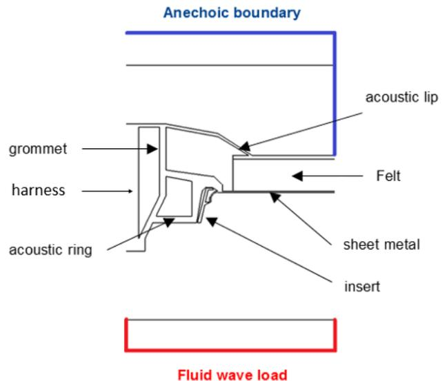
Figure 3: Materials, loading and boundary conditions of a dash grommet (cross-section).
