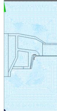
Figure 5: Mesh of the axisymmetric model of the small cabin with the wiring grommet (zoom).
