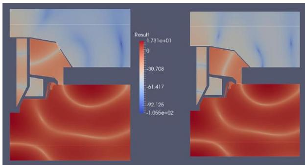
Figure 12: Acoustic pressure at 4000Hz for cavity length of 47mm (left) and 37mm (right).
