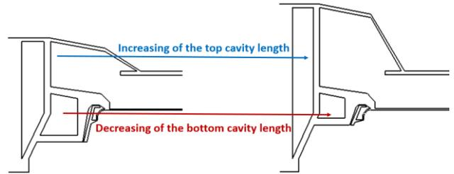
Figure 7: Example of geometrical configuration of a grommet.
