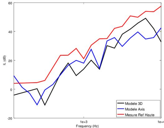
Figure 6: Measured IL (red curve) and computed IL for different models (3D model in black and axisymmetric model in blue) of the high reference.
