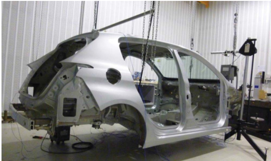
Figure 5: Suspended car body for dynamic measurements
